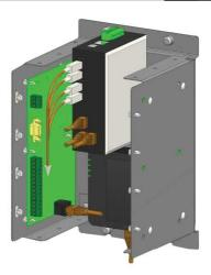
The QE20-FP2025 Fibre IP Networking Module, is used alongside the QE20-FP2005 RS485 Network Module to provide a fibre optic cable networking interface for a QE20 system. The fibre network consists of two fibres (TX and RX) wired in a ring around all the QE20 panels on the network. This kit can also be used as a replacement for an existing fibre module.
